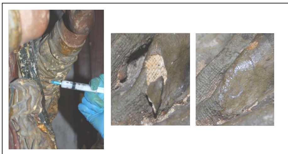
Figure 3. The re-adhesion of the ground layer involved applying 30% aqueous dispersion of Plextol B500.
